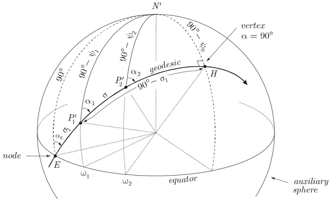
Figure 13: Geodesic on auxiliary sphere
