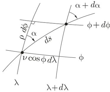
Figure 12a: Differential rectangle on ellipsoid
