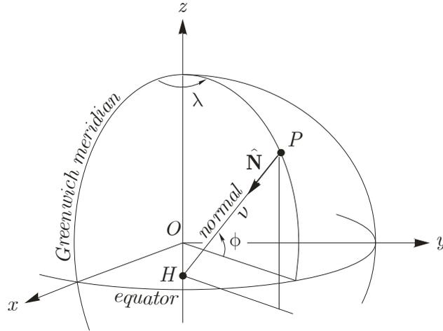
Figure 7: The unit normal  $\hat{\mathbf{N}}$  to the ellipsoid
