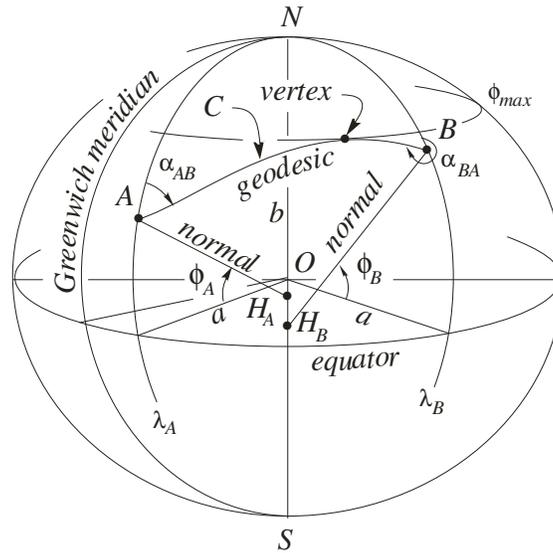
Fig. 1: Geodesic curve on an ellipsoid
