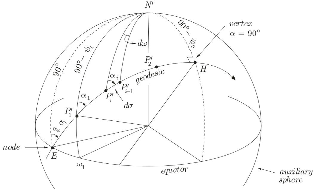
Figure 14: Geodesic on auxiliary sphere
