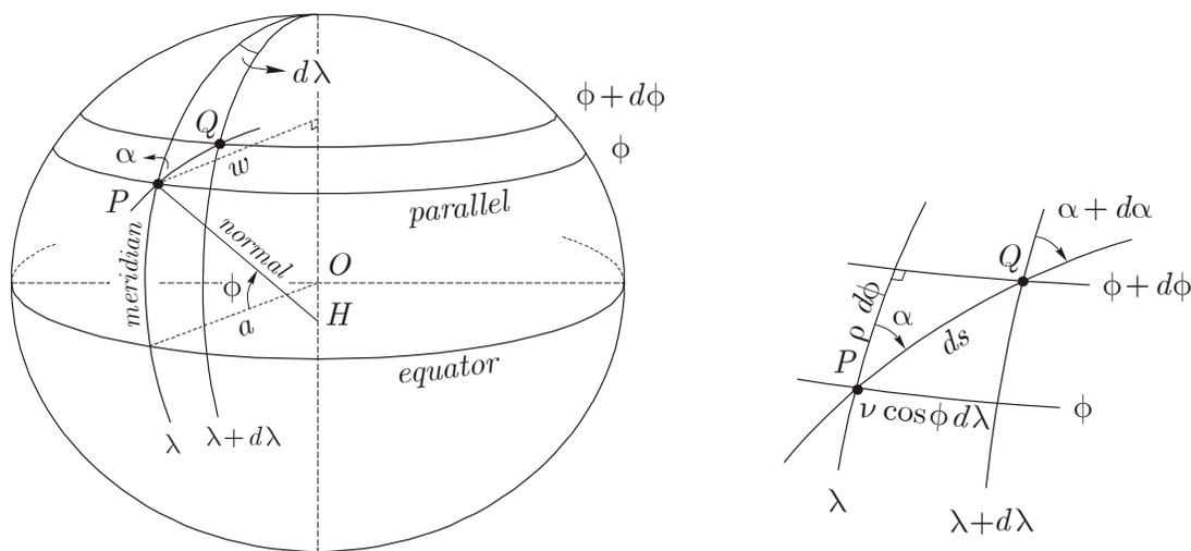
Figure 2: Differential rectangle on the ellipsoid
