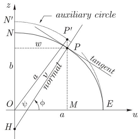
Figure 10: Meridian section of ellipsoid
