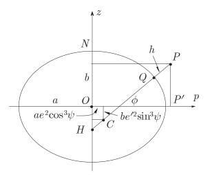
Figure 26: Coordinates of centre of curvature C
