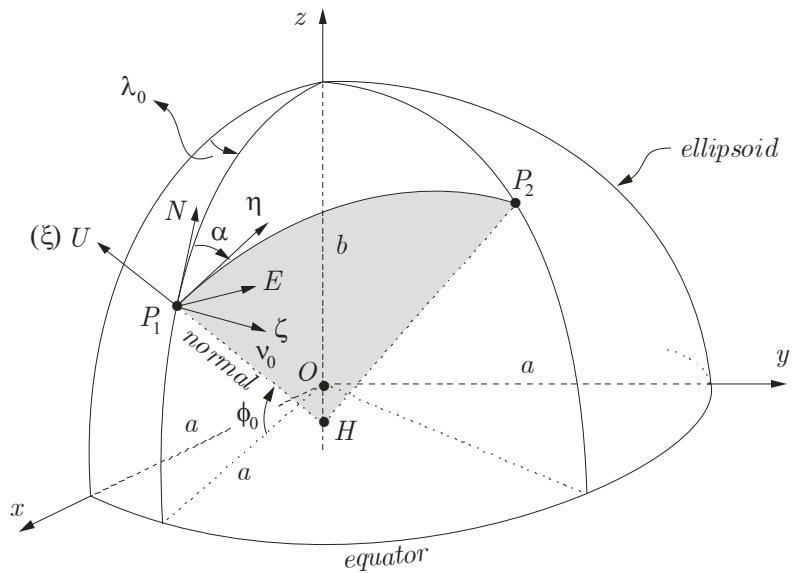
Figure 6: Rotated local coordinate system  $\zeta, \eta, \xi$
