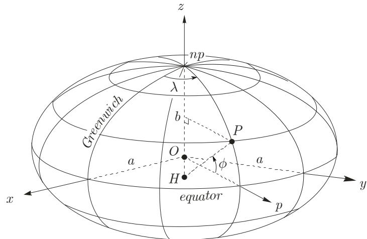
Figure 1: The reference ellipsoid
