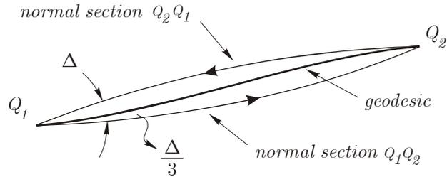
Figure 5. Geodesic curve between normal sections
