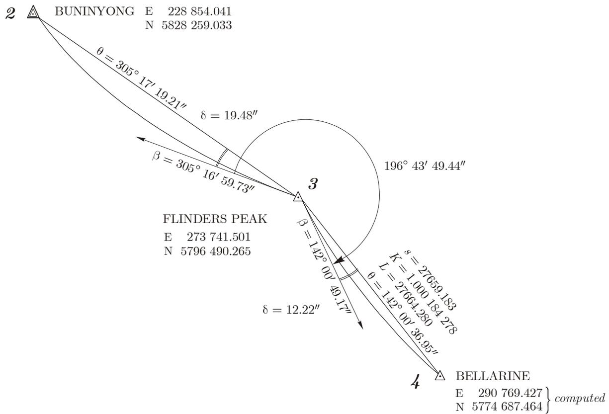
Figure 13 Traverse lines *Flinders Peak–Buninyong* and *Flinders Peak–Bellarine*.
