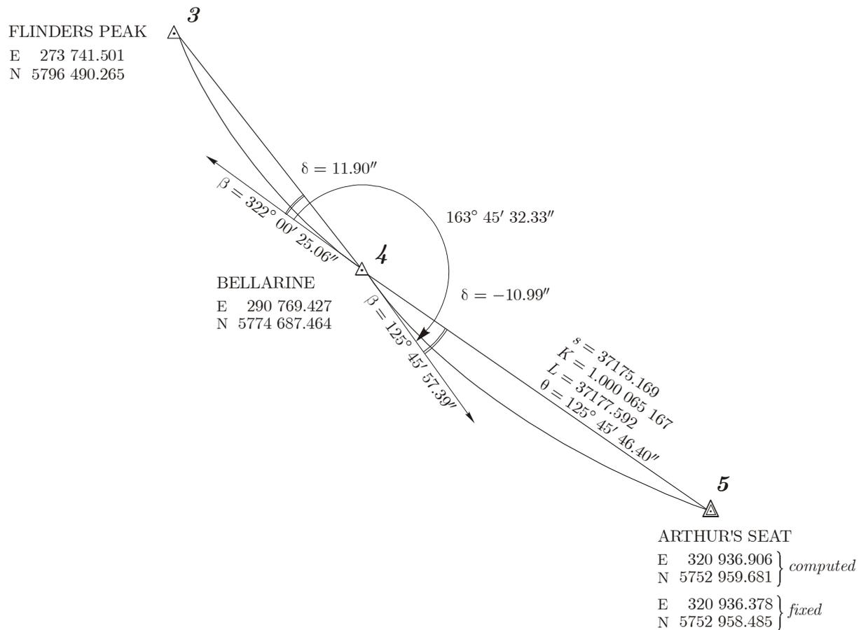
Figure 14 Traverse lines *Bellarine–Flinders Peak* and *Bellarine–Arthur's Seat*.
