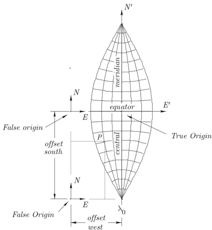
Figure 10 shows a schematic diagram of a UTM zone of the Earth. In the southern hemisphere the point  $P$  will have negative coordinates  $E', N'$  related to the true origin at the intersection of the central meridian and the equator.  $P$  has positive  $E, N$  coordinates related to the false origin 500,000 m west and 10,000,000 m south of the true origin. True origin and false origin coordinates in the southern hemisphere are related by
