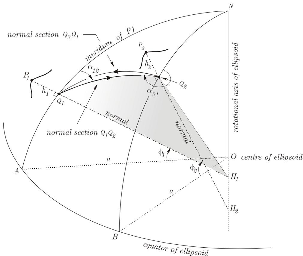
Figure 4. Reciprocal normal sections on the ellipsoid
