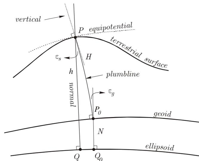
Figure 2. Projection of  $P$  on the Earth's surface to  $Q$  on the ellipsoid and  $P_0$  on the geoid. Note that  $P$ ,  $Q$ ,  $P_0$  and  $Q_0$  do not lie in the same vertical plane since the plumblines is a 3D space curve.
