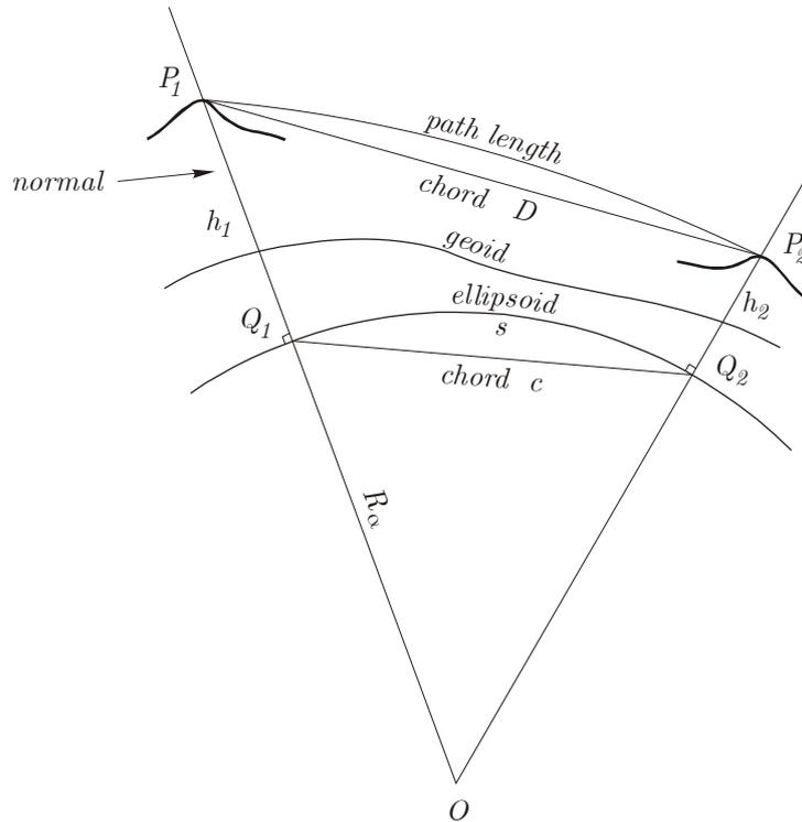
Figure 7. The geometry of the reduction of measured slope distances
