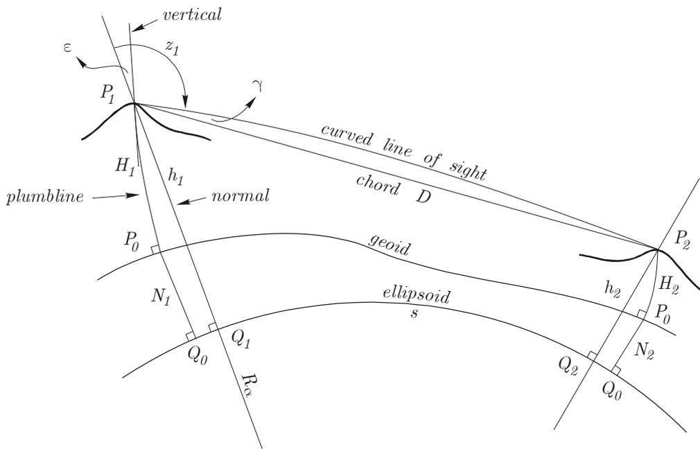
Figure 6. Zenith distance measurements and height differences
