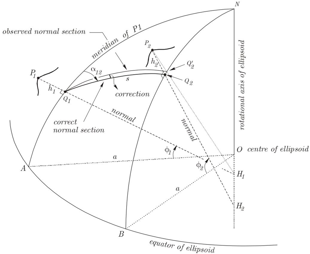
Figure 3. Skew-normal correction
